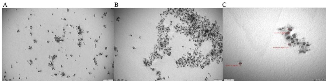
**Fig. 5** Transmission electron micrographs of biogenically synthesized silver nanoparticles at various magnification (60X, 100X and 150X), **(A)** Low-magnification TEM image showing the overall morphology and dispersion of nanoparticles. **(B)** Higher magnification image displaying the internal structure and boundaries of the nanoparticles. **(C)** Further high-resolution TEM image revealing the atomic arrangement within the material
